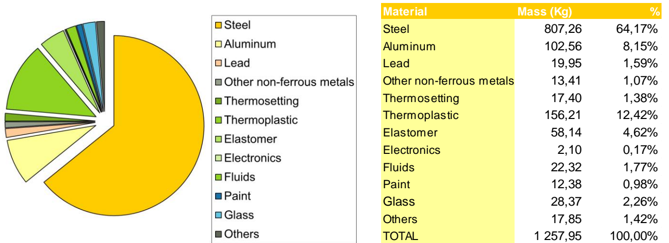
Figure 13: Material composition of Fluence, 1,6l 16v petrol engine
